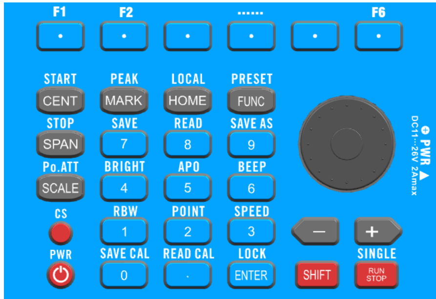
Figure 3-1: Keyboard of KC901x
