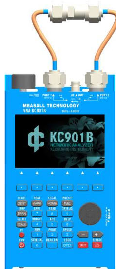
Figure 4-2: Calibration connection when testing with two cables
