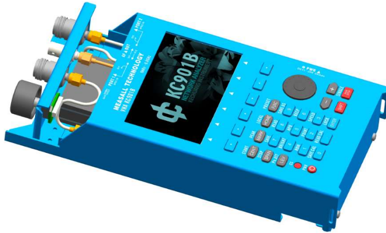
Figure 2-2, step 2, slide the upper cover towards the end about 2 cm
