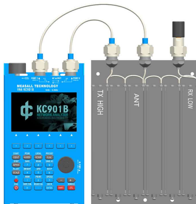
Figure 5-1: Example of test duplexer connection method
