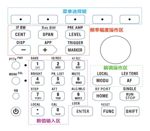
For quick operation, The common menu function set to the second layer key, press SHIFT key to access. Following is the first layer of keyboard:
