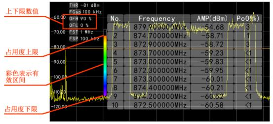
(8) After a period of time, check the **PEAK TABLE** and estimate whether the signal of interest is logged. If the answer is yes, press the save button on the soft menu to save the table.
