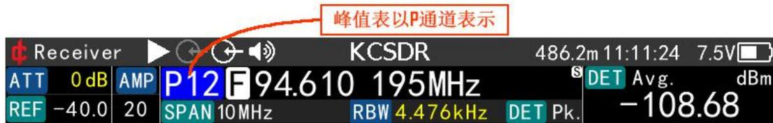
No matter where the frequency comes from, channel or peak list, **user should push it to VFO** if user wants to adjust the parameters temporarily.
