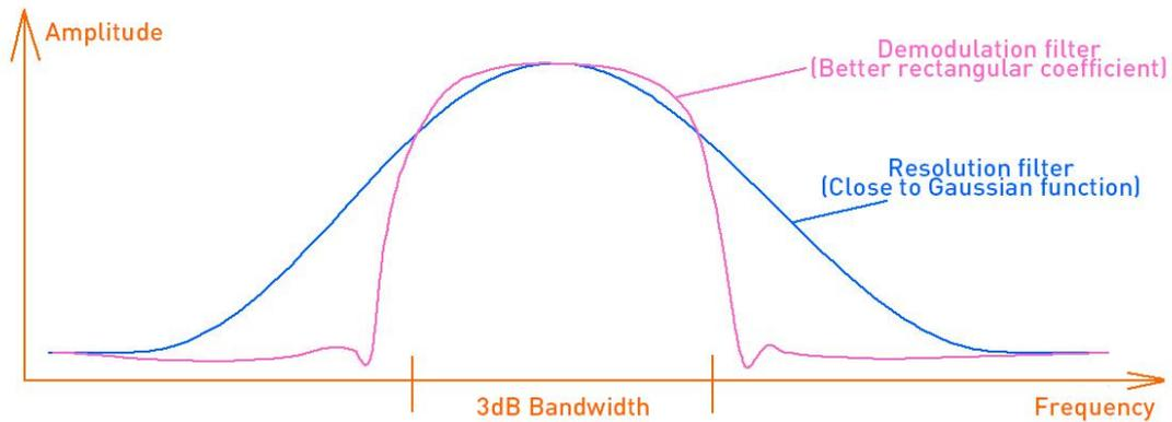
For wide-band signals, the wider the resolution bandwidth or demodulation bandwidth is set, the larger the readout will be.
