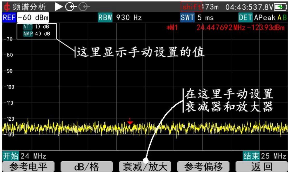
Vice versa, switching AMP off or increasing ATT value cannot reduce the interactive interference within the machine, yet it might even become unneglectable without the amplifier's noise.
