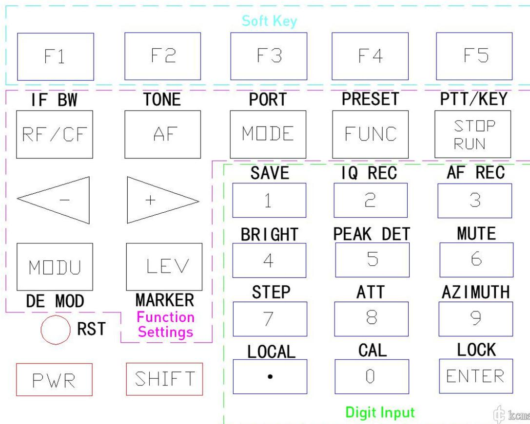
For quick operation, The common menu function set to the second layer key, press SHIFT key to access. Following is the first layer of keyboard:
