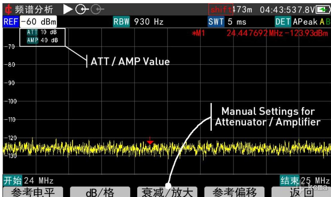
KC908 has been tuned for optimal performance while being used with hand-held antenna. Under ideal electromagnetic environment, setting ATT
