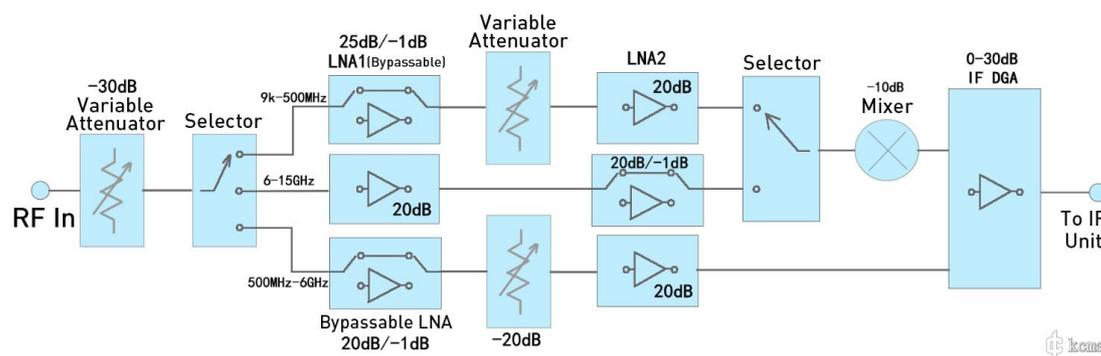
The gain of the IF amplifier can be numerically controlled, which is done automatically. And the range is 0-30dB. To sum up, a maximum gain of 70dB can be achieved with amplifier combination in the front of ADC. Take the loss
