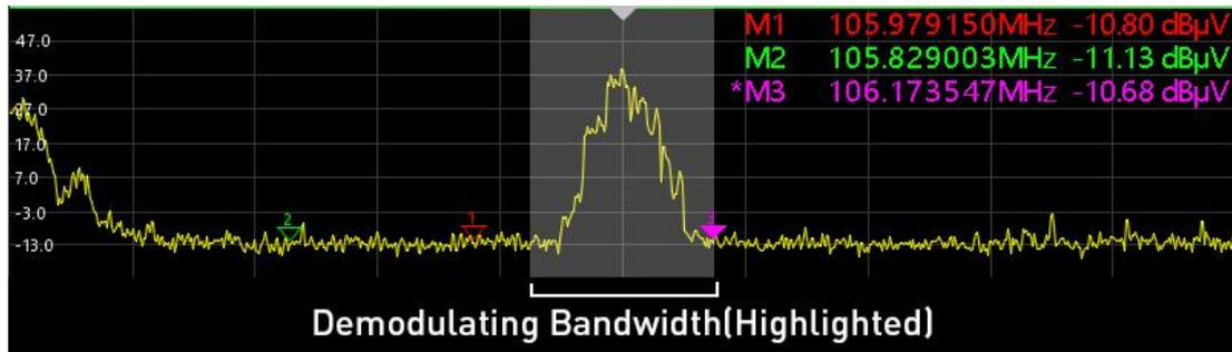
In **MODU** menu, **DETECTOR** defines the way level meter detects the signals. This setting can be neglected if the user just want to take a glance of the level/field strength. Whereas a precise field strength measurement demands the **DETECTOR** parameter properly set according to different modulating methods of the signal, or according to relevant standards.
