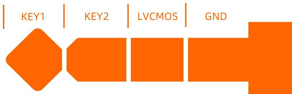
KEY1 and KEY2 are used to connect the telegraph key. While using a manual key it should connect to KEY1 and GND. To use an automatic key user should connect KEY1, KEY2 and GND. The driving voltage for key is usually 1.8V.
