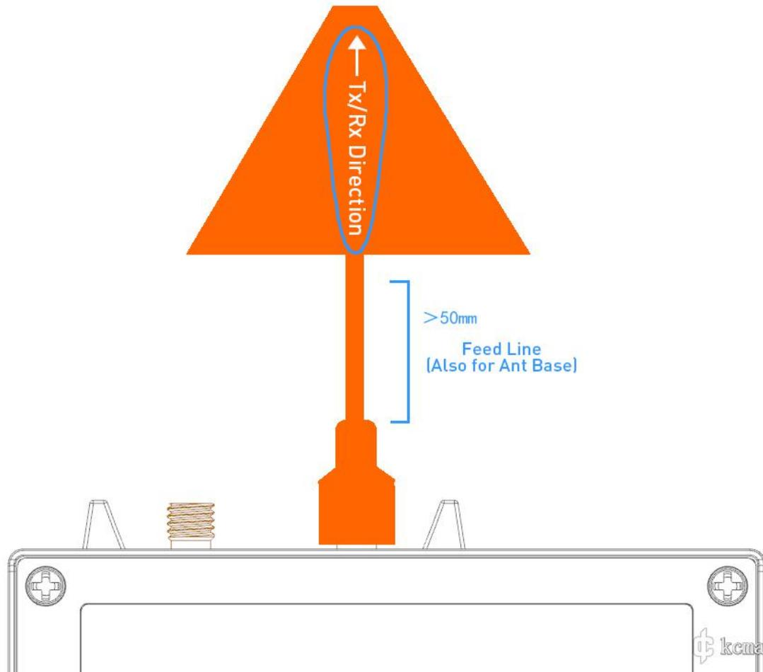
(4) The root of the handle of the antenna should be firm. Otherwise the core pin would tend to waggle, consequently damaging the RF port.
