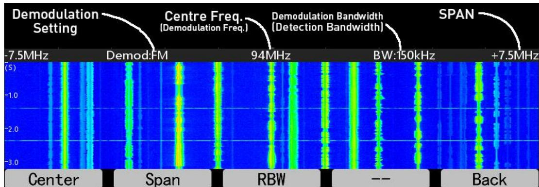
(14) Adjust the antenna , find out the position and direction where field strength maximizes and watch the reading on the screen. For screenshots, press SHIFT+1.
